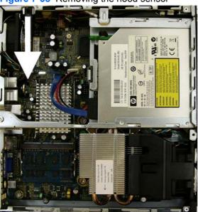
Figure 7-38 Removing the hood sensor
